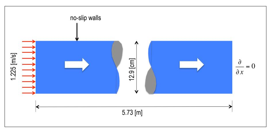
Working fluid = AIR Kinematic viscosity = 1.58 E-05 Reynolds number = 31,577
