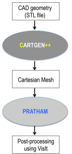
Fully parallel mesh generator C++ with MPI
