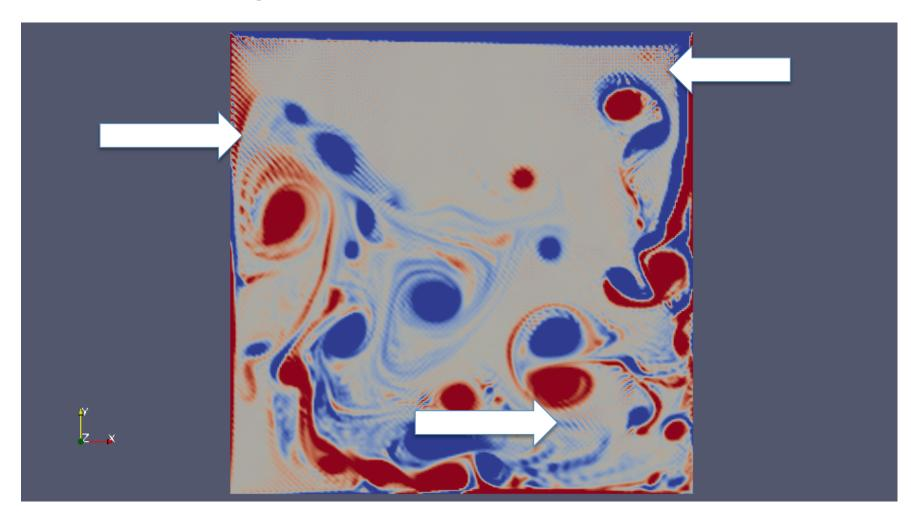
Note the oscillations in the solution at various places. This is possibly because of the BGK collision term employed. A movie of this simulation can be seen at the following link:
