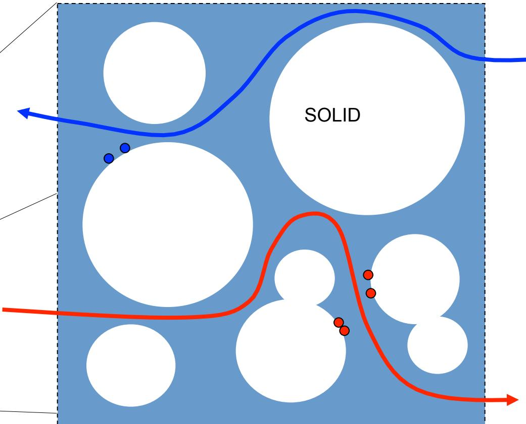
Chemical reactions among gas components need to be included for the case of internal reforming and at the TPB.
